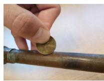
Copper pipe Magnets do not stick to copper pipes.
