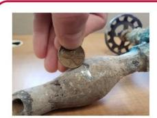
Lead pipe Magnets do not stick to lead pipes.
